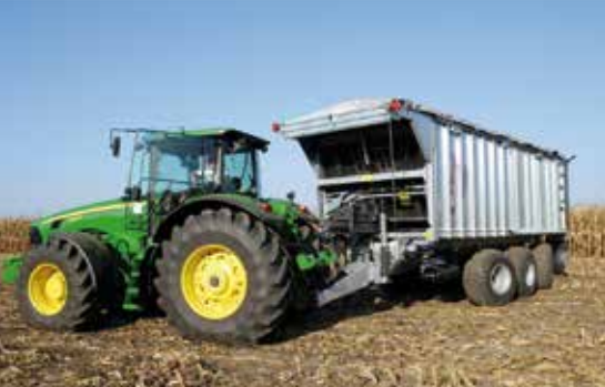
Electronic Forced steering »ForCon 2010«. Contactless drive, resulting in no steering limit (option).
